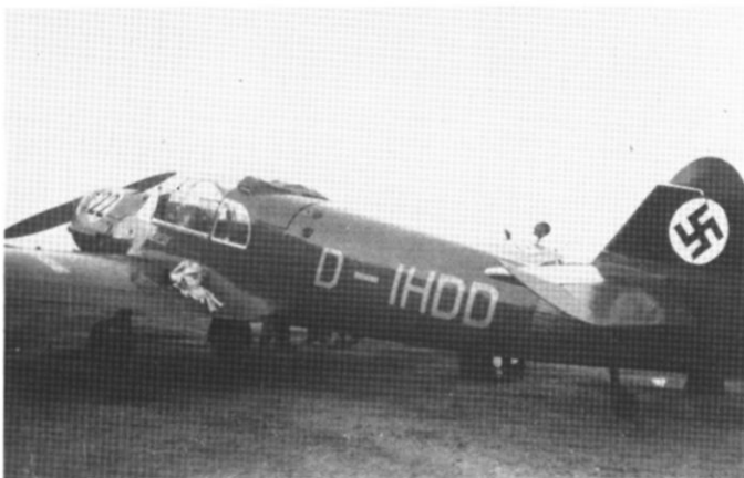
Left. Some Messerschmitt Bf 108s received an overall coat of blue-black paint which was highly polished. This one had the civilian registration D-IHDD marked in cream 05, a competition number on the nose, and the usual text stencilled in black on the rear fuselage. The cockpit framing was left in bare metal, a common practice. Right. An unusual code was used on this liaison Fieseler Fi 156 used by an unknown officer. The letters FIME were painted aft of the fuselage cross and also on the upper surfaces of the wing. A standard 70/71/65 color scheme was used.
