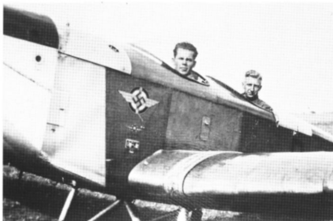
Left. In the paramilitary NSFK or National Socialist Flying Corps the aircraft were simply varnished to protect the plywood parts. Such was the case with this Klemm K1 25 which also had its engine cowling in bare metal except for the black upper panel from another aircraft. Above the manufacturer's construction plate was the Klemm factory emblem which, in turn, was surmounted by a variant of the NSFK insigne. Right. On the Klemm K1 25 the plywood parts not requiring covering were usually varnished instead of being painted, such as is seen here on these aircraft of the FFS at Herzogenaurach during 1937. Other parts of the aircraft were painted silver, the engine cowlings being left in bare metal.
