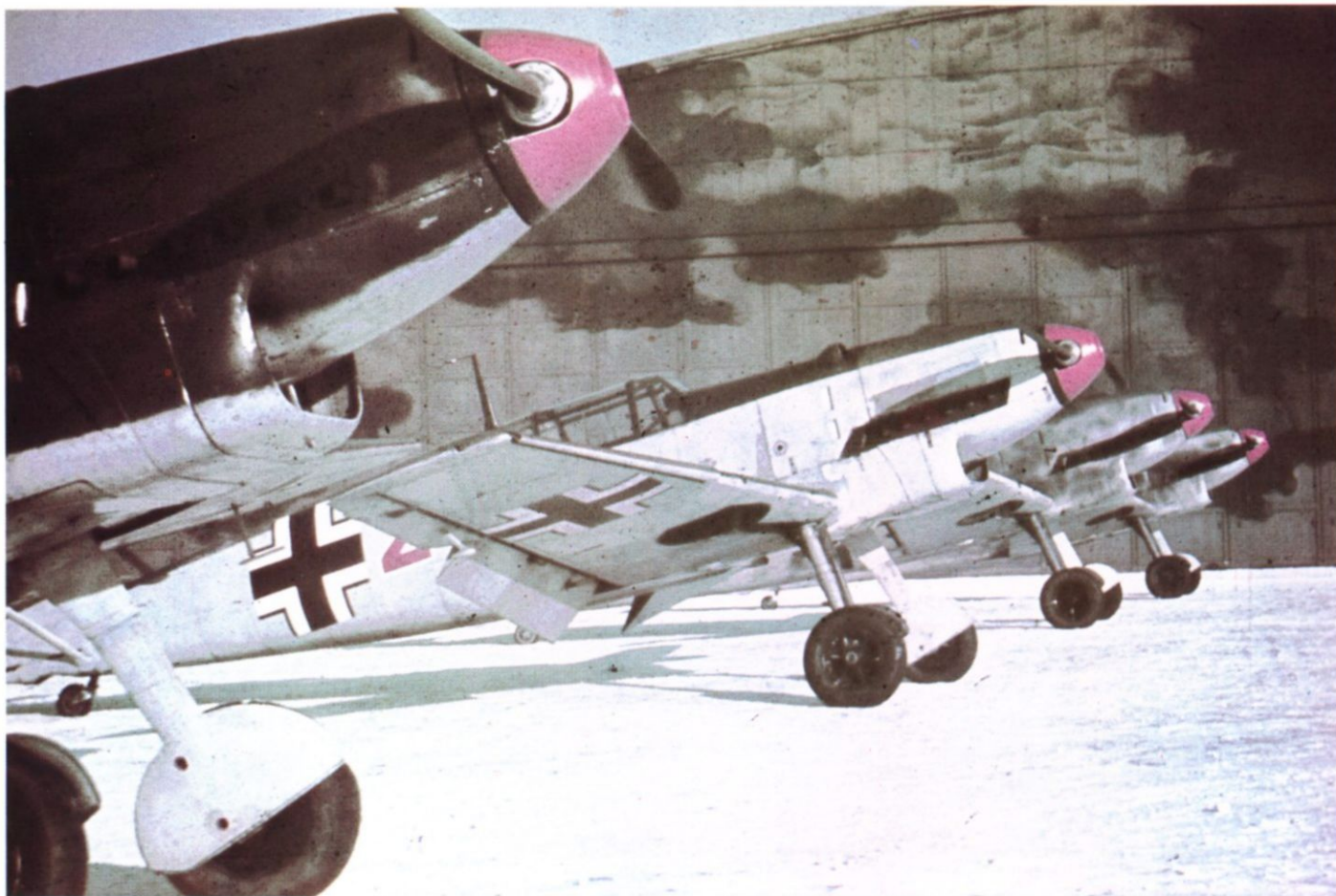
Upper. A line-up of four Bf 109Cs at a fighter training school in Germany in late 1940. Three distinctive styles of camouflage are evident, the aircraft on the left having the pre-war greens 70 and 71 right down the fuselage sides with the usual pale blue 65 undersurfaces. The middle aircraft had the same colors but with the raised color separation line as used in the French campaign. The last two show a random overspray over their pale blue fuselage sides to provide a better camouflage effect when dispersed on the ground. The glossy pink paint – not faded red – used for the spinners and identification numbers was probably a mixture of roughly equal parts of red 23 and white. Lower. An interesting photograph taken on 30th June 1939 showing a newly completed Minimoa sailplane in the NSFK color pale cream with clear doped fabric surfaces. The blown canopy is of interest.
