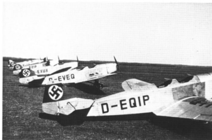
Left. In the paramilitary NSFK or National Socialist Flying Corps the aircraft were simply varnished to protect the plywood parts. Such was the case with this Klemm K1 25 which also had its engine cowling in bare metal except for the black upper panel from another aircraft. Above the manufacturer's construction plate was the Klemm factory emblem which, in turn, was surmounted by a variant of the NSFK insigne. Right. On the Klemm K1 25 the plywood parts not requiring covering were usually varnished instead of being painted, such as is seen here on these aircraft of the FFS at Herzogenaurach during 1937. Other parts of the aircraft were painted silver, the engine cowlings being left in bare metal.
