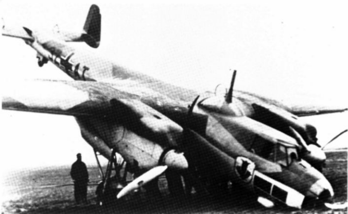
Left. Formed in late 1937, 2./Kü Fl Gr was based at Dievenov. Equipped in 1939 with the Dornier Do 18, the Staffel retained the old registration for a considerable time. This shot shows the standard finish for flying boats; all surfaces visible when the aircraft was in the water were painted RLM grey 02, the undersurfaces of the hull and sponsons being covered with a coat of silver 01 plus two coats of clear lacquer. The Staffel unit emblem appeared on both sides of the engine cowling, and by this time the red horizontal fin and rudder band had vanished. Right. More careful use of the brakes might have prevented this landing accident to 3Z+AT, a Do 17 of the Alpen Geschwader , KG 153. It bore the Gentian emblem which became the insignie of the first two Gruppen of KG 255. It was camouflaged in the usual four colors and had bare metal propeller blades and yellow spinners.
