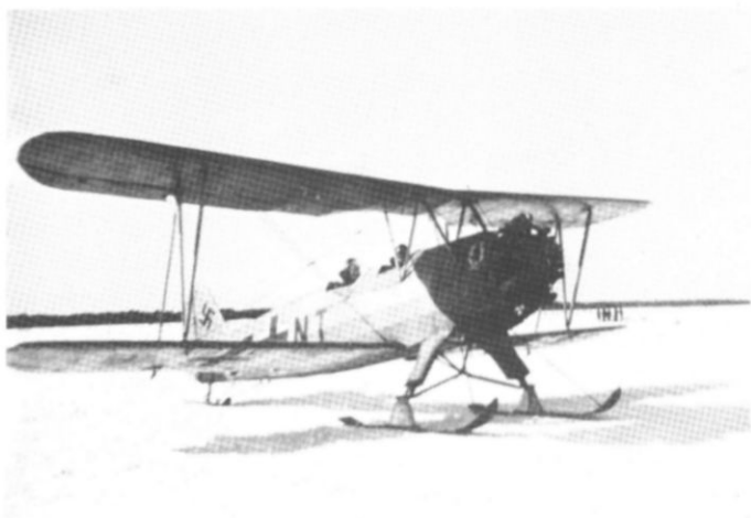
Left. Some Focke-Wulf Fw 44 Stieglitz trainers were fitted with skis, this one being finished in overall RLM grey 02. Just behind the engine was an unidentified unit badge. Can any reader identify the unit? Right. Another Stieglitz , this beautifully clean example was photographed just before take-off from Pilsen in 1940. The non-regulation fuselage cross had still not been modified and in this case the finish was overall silver.
