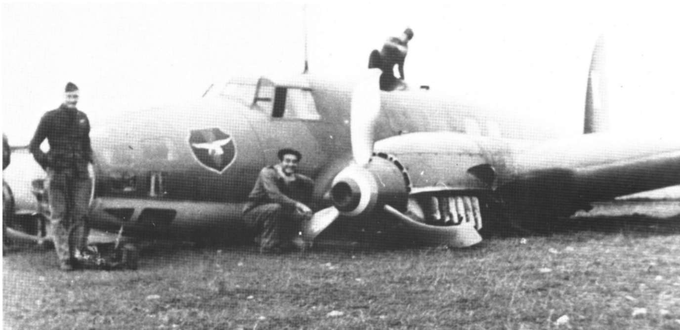
This crashed Heinkel He 111 shows an early version of what was later to become the insignia of IV./KG 53. The upper surface three-color camouflage had faded somewhat in intensity. The white letter K on the fin is of interest for this was an unusual practice at the time. Bare metal propeller blades are visible here and the three-color spinner may have been red, yellow and red, the colors of Nationalist Spain.
