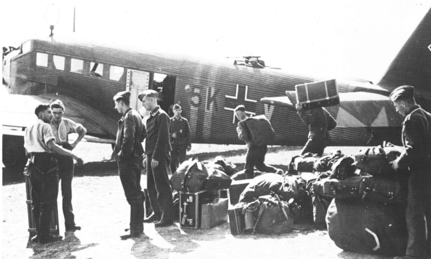
Upper. Another transport aircraft attached to a bomber unit, in this case KG 3 Blitz Geschwader . This long-serving "Auntie" had its old three-tone camouflage overpainted in standard 70 and 71 but it is still possible to discern grey parts on the elevator and the two yellow bands under the 5K of the code, showing that this particular aircraft had served previously in a blind flying school. Lower. Can anyone identify the unit indicated here by the prefix B1? This Junkers W 34 managed to stand on its nose after landing on a soft grass runway. Painted RLM grey 02 overall, it carried the oversized upper surface wing crosses introduced after the Polish campaign. Interesting details for the modeller are the electric generator, the large radio mast, the loop antenna and tailskid.
