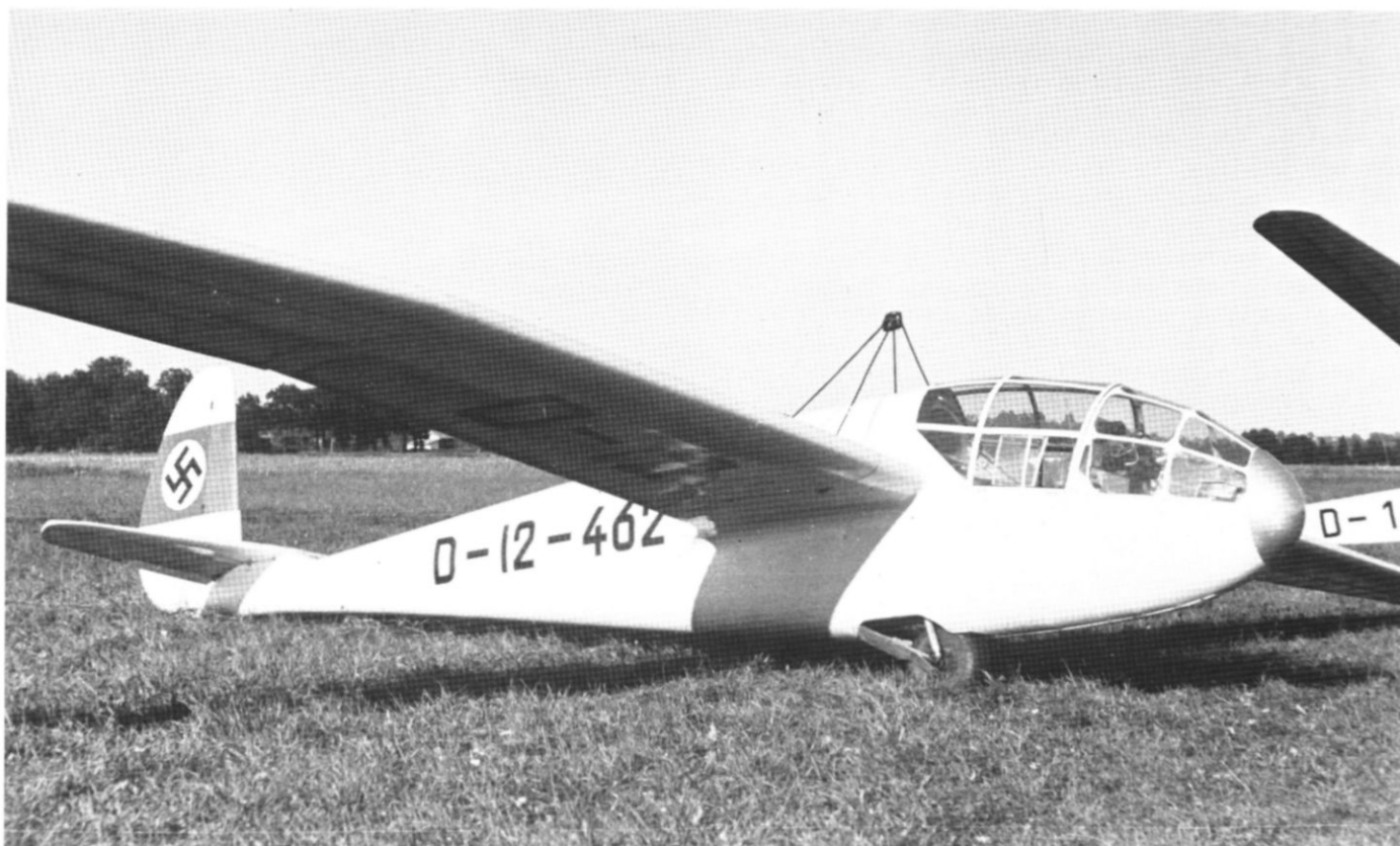
Upper. The quest for high performance gave rise to some elegant sailplanes, of which the FVA 10b Rheinland was one. It won the award for advanced technical design at the 1937 Rhoen competitions, its fuselage shape being designed to conform as closely as possible to the airflow over the wings. Its landing wheel was made semi-retractable and the nosecap was painted red. Finish was the usual glossy pale cream. On this example the registration was rather smaller than was normal. Lower. Illustrating three distinctly different color schemes, this photograph shows a partly assembled Condor II in varnished wood and clear doped finish but no registration, a two-seat Göppingen 4 II , D-13-436 in overall pale cream, and a Habicht , D-8-51, in the colorful pale cream and medium blue sunburst aerobatic scheme also shown on another machine on Page 53.
