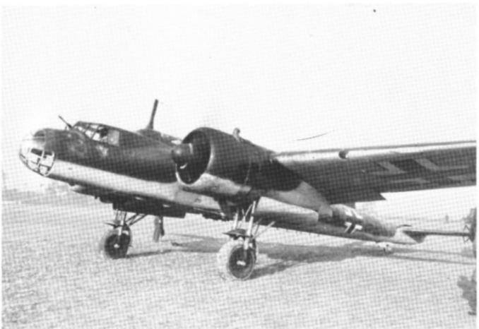
Left. Although 3.(F)/11 used mainly Messerschmitt Bf 110s during the Battle of Britain, it had some Dornier Do 17Ps such as 6M+GL shown here. Wearing standard 70/71/65 camouflage, it still showed faint traces of its previous three-color camouflage around the cockpit area. A feature rarely seen in photographs is the rack under the fuselage for four small flare bombs. Right. A Messerschmitt Bf 110, U8+BL, preparing to take off from Yvrench airfield in northern France in 1940. It wore the newly-introduced 71/02 camouflage but retained a thin white band around its rear fuselage. The nose had also been overpainted in white as a recognition aid.
