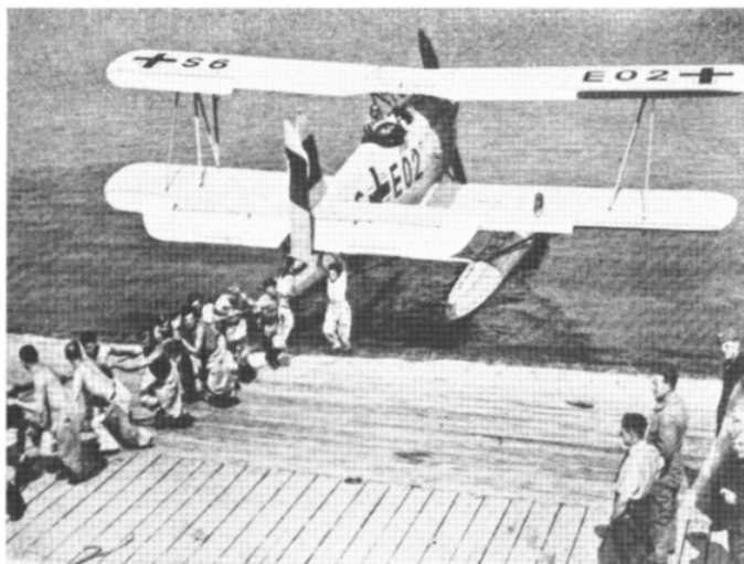
Left. This Heinkel He 60 was being pulled onto the slipway after completing a flight. The required RLM grey 02 finish appears lighter than usual and was probably closer in shade to pale grey. On this aircraft a camera gun was mounted on the bottom starboard wing. Both floats were probably silver. Right. Temporary black paint covered all the undersurfaces of this Junkers Ju 86 used by Blindflugschule 2 in Neuberg during 1939. The interesting emblem under the cockpit was the head of a white cow!
