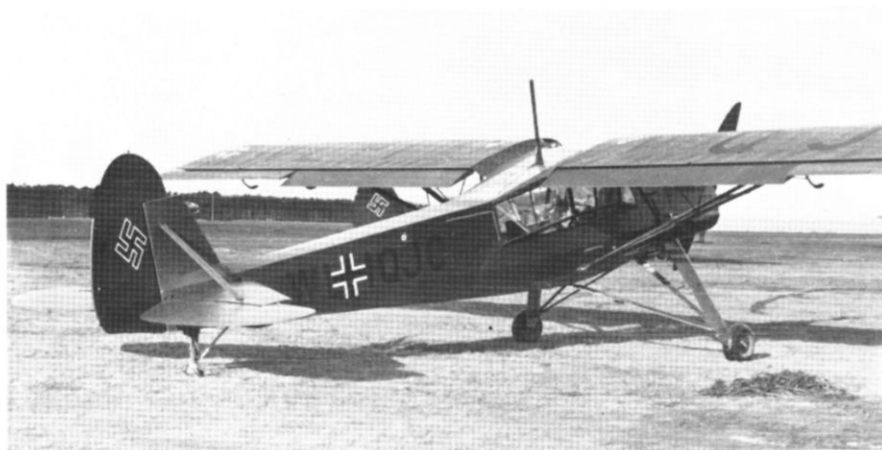
Left. On this Fieseler Storch, WL+IQJC, the fuselage cross was literally jammed in between the letters L and I of the registration and the upper wing crosses were quite small. The contrast between the two shades of green, 70 and 71, was only just discernable. The small white spot and tiny red cross between the Q and the J indicated the position of the medicine chest. Right. The twenty-first aircraft of the flying school at Grossenhain-Dresden in 1936, this Heinkel He 45 was about to take off. Painted overall greenish-grey 63, it carried the registration system introduced in June 1936.
