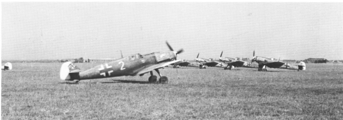
Showing the Bonzo mascot on their cowlings, these Messerschmitt Bf 109s of 1./JG 2 had the same type of camouflage and white tactical markings on their rudders and wingtips. In this shot it is obvious that the former white engine cowlings had been lightly camouflaged. The spinners, however, were overall white. The photograph shows the old style of fuselage cross still in use even in the second half of 1940.
