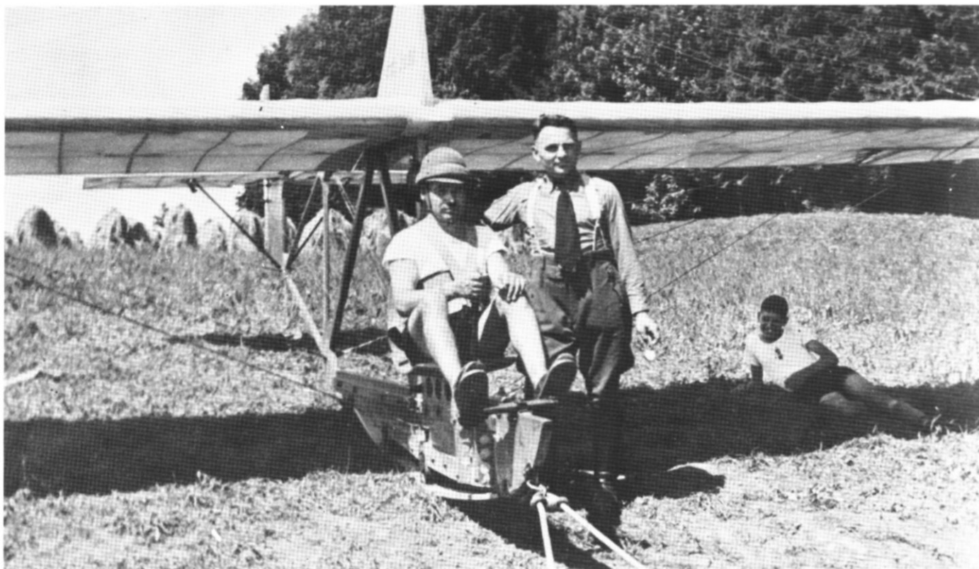
Bungee cords taut, a trainee pilot prepares to be catapulted into space in an SG 38 primary glider. The machine was named Ernst Huchel in memory of a respected instructor killed in a flying accident. Holding the stopwatch preparing to record the flight time is Konrad Dehn, another flying instructor.
