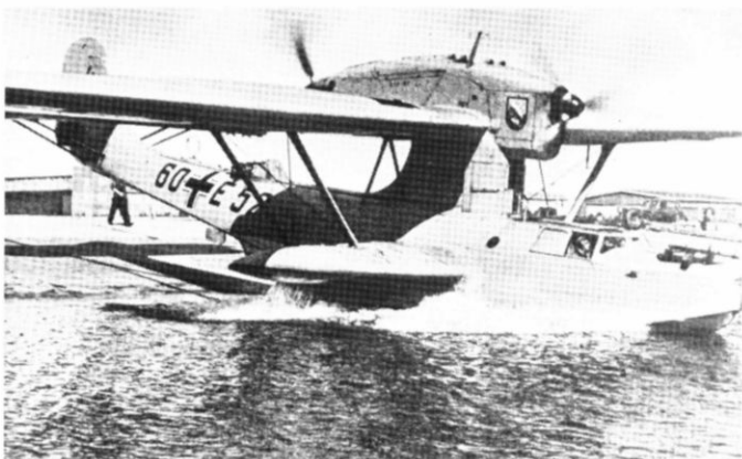
Left. Formed in late 1937, 2./Kü Fl Gr was based at Dievenov. Equipped in 1939 with the Dornier Do 18, the Staffel retained the old registration for a considerable time. This shot shows the standard finish for flying boats; all surfaces visible when the aircraft was in the water were painted RLM grey 02, the undersurfaces of the hull and sponsons being covered with a coat of silver 01 plus two coats of clear lacquer. The Staffel unit emblem appeared on both sides of the engine cowling, and by this time the red horizontal fin and rudder band had vanished. Right. More careful use of the brakes might have prevented this landing accident to 3Z+AT, a Do 17 of the Alpen Geschwader , KG 153. It bore the Gentian emblem which became the insignie of the first two Gruppen of KG 255. It was camouflaged in the usual four colors and had bare metal propeller blades and yellow spinners.
