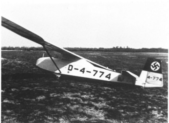
Left. What's this? Nothing more than another Wolf with a Grunau Baby's rudder, a component very similar in area but of different shape and only partly painted pale cream like the rest of the aircraft. Right. Capturing all the thrill of silent flight, this overall pale cream Minimoa heads out across a valley after being catapulted off by its rubber bungee cord and helpers. The registration was painted above and below the wings.
