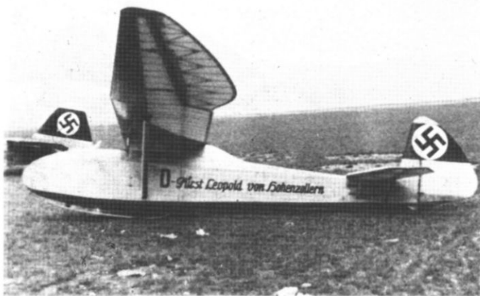
Left. This 1935 photograph shows the second Wolf produced. The entire aircraft had a clear doped and varnished finish except for the lettering and national markings. It is highly likely that the starboard fin and rudder would have carried the red, white and black national colors. The legend under the tailplane seems to read: TYP — WOLF Sport — Flugzeugbau Göppingen. Right. Photographed in 1936, this is another sailplane of the same type, appropriately enough bearing the registration D-WOLF on the fuselage and showing its aerobatic markings to perfection. The color scheme was pale cream and medium blue. The trim and entire elevator appears to have been medium blue.
