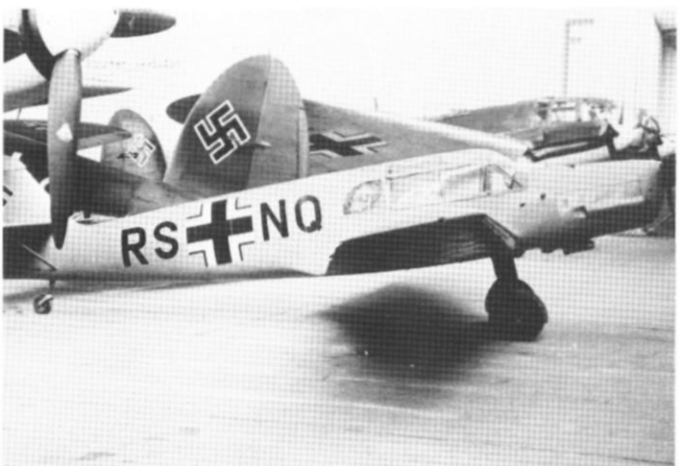
Left. Photographed in 1940 amongst Heinkel He 111s of KG 53, this Messerschmitt Bf 108 was used by the unit as a liaison aircraft. Painted overall RLM grey 02, it wore the "second generation" type of fuselage cross with the swastika in the early rearward position. Note the tiny red cross within the usual white disc under the letter N of the code and the VDM manufacturer's triangles on the propeller blades of the Heinkel in the foreground. Right. This old Junkers Ju 52 was used as a transport by KG 3 and carried the code 5K+VM. Even then, in 1940, it retained its old 61/62/63/65 camouflage and early style of national markings. The red band and white disc under the swastika had obviously been repainted in dark green.
