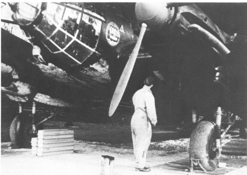
Taken in France in 1940, this photograph demonstrates clearly that the quality of the camouflage paint, even at the beginning of hostilities, left much to be desired. After several flights over Britain, this Heinkel He 111 of 1./KG 100 had lost much of its temporary black undersurfaces and required retouching. The colors of the framing around the nose are interesting.
