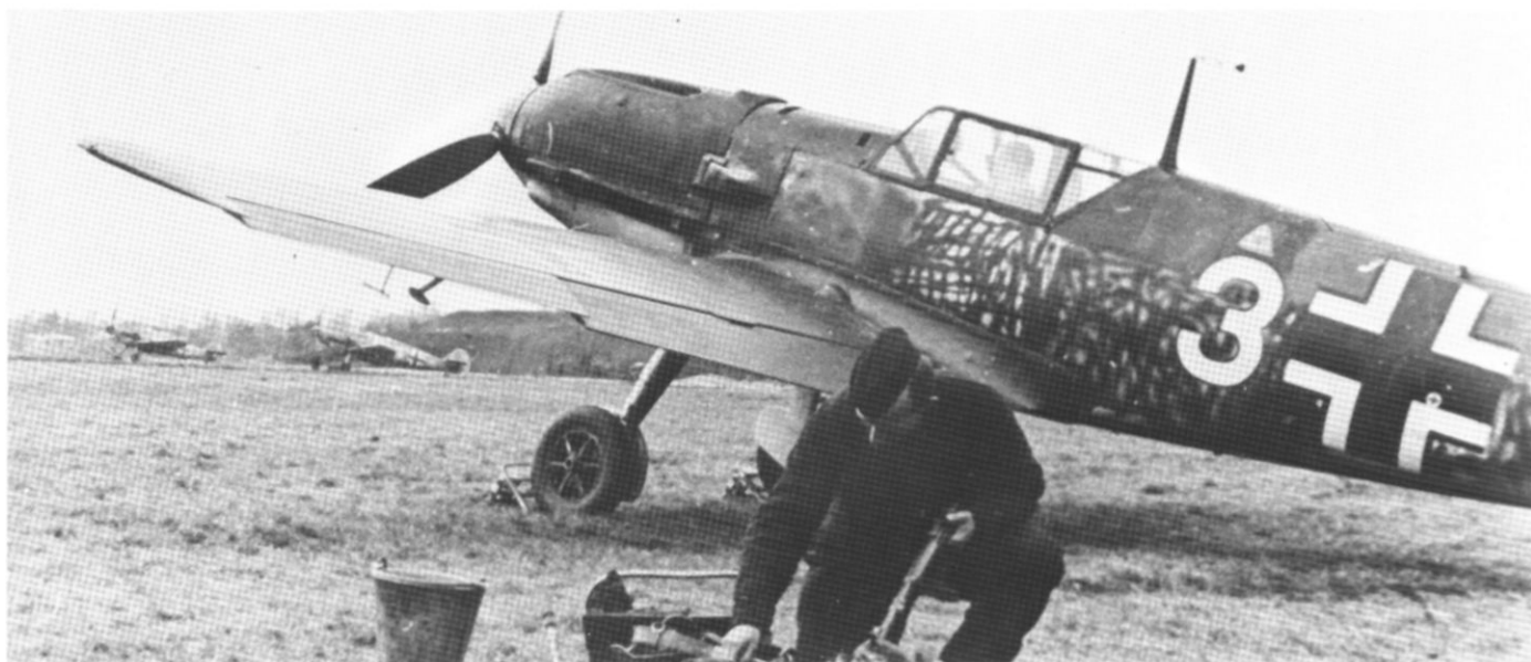
Upper. In late 1940, operational fighters received many kinds of field camouflage yet on this example the dark green 71 additions to the fuselage were still decidedly unusual. The low dividing line of the topmost fuselage colors was rather uncommon. Lower. After being badly hit on a mission over England, this Junkers Ju 88 just managed to make it back to France. All the undersurfaces and fuselage sides were painted black except for the white parts of the crosses and swastika. On the original photograph it was possible to see a white letter E on the upper starboard wingtip. The bomber belonged to 1./KG 51 Edelweiss .
