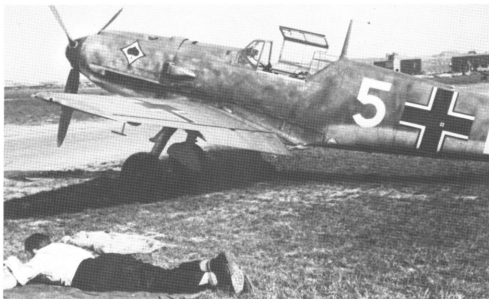
The pale blue fuselage sides of the Messerschmitt Bf 109E-3s of 7./JG 53 were completely overpainted using large applications of the colors 71 and 02. Even when this photograph was taken in France in Summer, 1940, the early type of fuselage cross was still in use.
