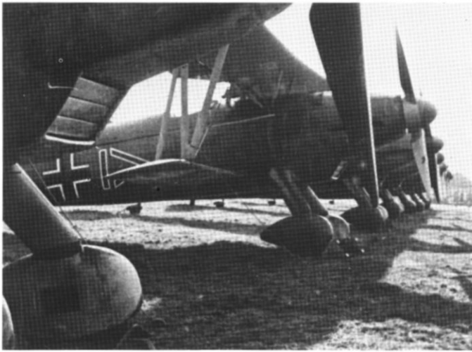
Left. Taken in September 1938, this photograph shows one of the first applications of the dark greens 70 and 71 with pale blue-grey 65 camouflage. The second Arado Ar 68 wore the chevron and bar symbol of the Geschwader Adjutant . Right. This photograph shows that even the replacement of a simple panel can change a pattern as it has under the fuel triangle of this Arado Ar 68. The angry cat emblem dates from the pre-war period and was even to be seen on the engine cowlings of some Fw 190D-9s in 1945.
