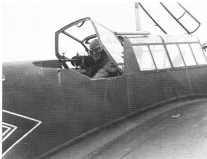
Left. A close-up of the rear fuselage of a 4./KG 55 Heinkel He 111 showing all the light parts overpainted in temporary black for night missions. The thin white outline of the letter D had even been included in this process. Right. Especially interesting to the modeller, this shot shows the cockpit area of a Messerschmitt Bf 110 with all hatches open. The contrast between the 70/71 camouflage is barely discernable and the double chevron of the Gruppe Kommodore of I./ZG 76 was simply outlined in white on the fuselage. The lower part of the radio mast was painted yellow.
