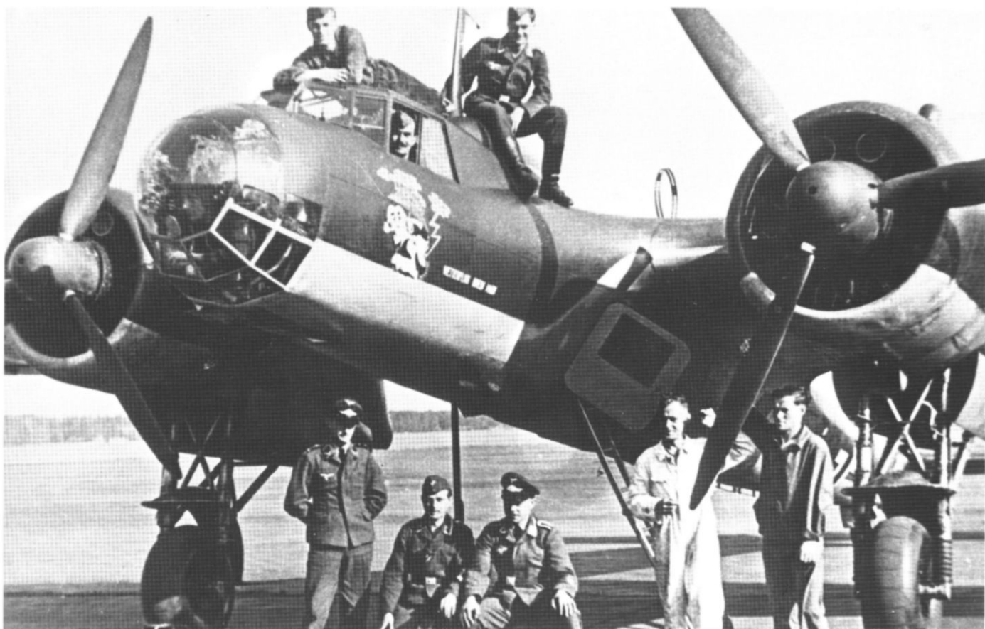
Upper. Good photographs of Luftwaffe aircraft serving in weather units are rare. Unfortunately the code of this Dornier Do 17P is not known but its emblem followed by the words Wetter Flug Rhein-Main (Rhein-Main Weather Unit) is of interest. The aircraft had standard 70/71/65 camouflage with black-green propeller blades and spinners. Uffz Jakob Mitschke was seated in the centre. The photograph was taken in 1939. Lower. Waiting for action. This Heinkel He 111 of the ninth Staffel of III./LG I had quite battered camouflage after only a few weeks of operations, suggesting that the dark green 71 especially may not have been of a very high quality in 1939. Its yellow spinners indicated the third Gruppe . The fuselage and lower surfaces of the wings wore old-style crosses and the large exhaust marks are very obvious.
